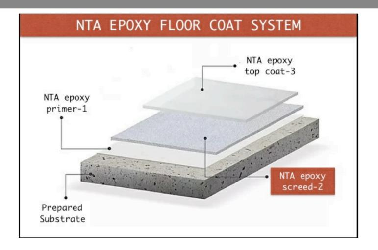
Epoxy self levelling screed HIGH PERFORMANCE, EPOXY RESIN FLOORING SYSTEM, SUPPLIED AS THREE PARTS IN A PREMEASURED PACK FOR EASE OF ON SITE MIXING AND USE. THE CURED RESINS FORM A SMOOTH, TOUGH 2-4 mm LAYER, WHICH CAN BE EASILY CLEANED
