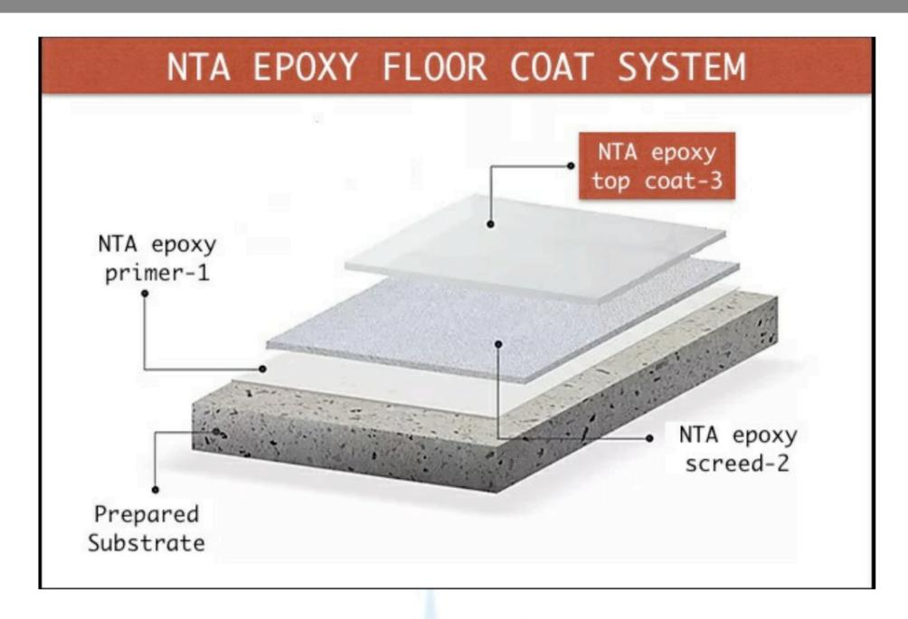
Self-smoothing epoxy floor system with high performance, supplied in four part in a pre-measured pack to provide ease in the usage at on-going sites with high performance, supplied as four parts in a premeasured pack for ease on site mixing and use. The cured resins form a pigmented, smooth, tough 2-4 mm layer, which can be easily cleaned.
